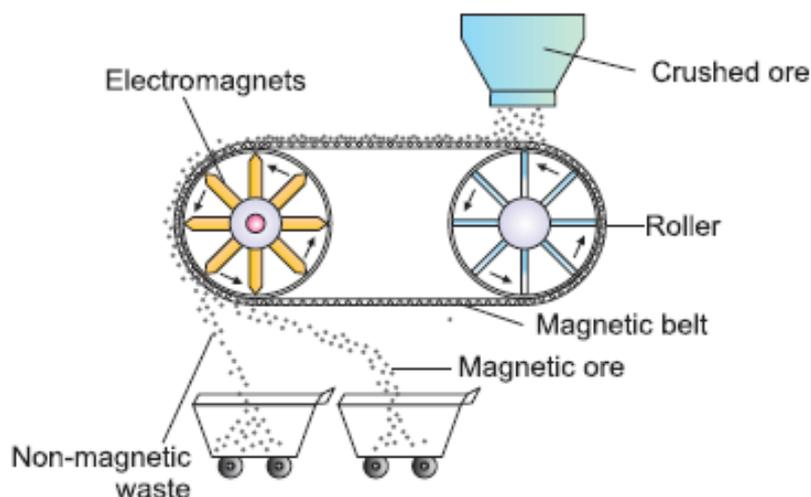
Fig 16.3: Magnetic separation
