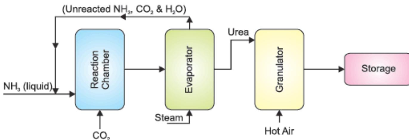
Fig. 16.9 Flow sheet diagram of Urea
