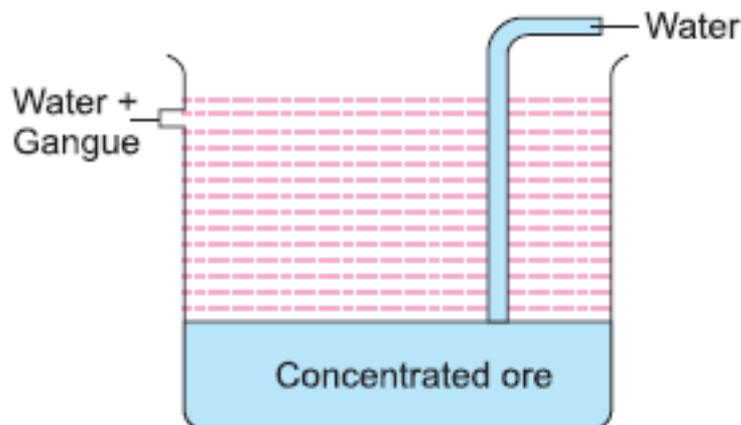
Fig. 16.1 Gravity separation
