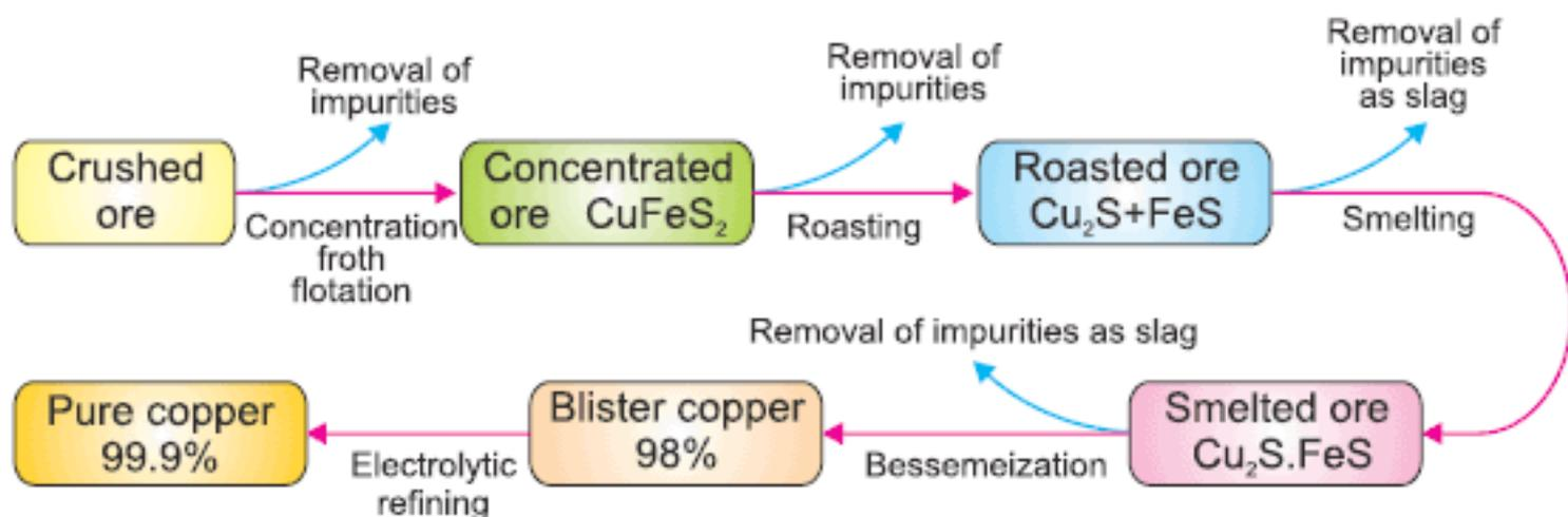
Fig. 16.7 Flow sheet diagram for extraction of copper
