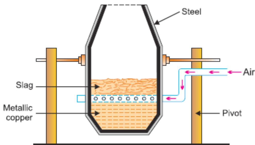
Fig. 16.5 Bessemer converter used for bessemerization of copper.
