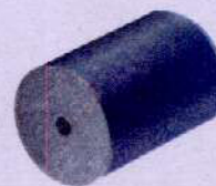
Figure 6.19: Nuclear fuel pellets used in nuclear reactors.
